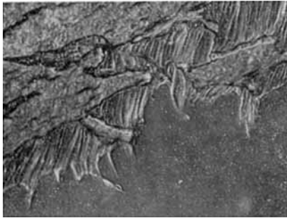
Fig. 5. Fracture edge of an unnotched sample stressed in igepal. Phase contrast, 70X.
